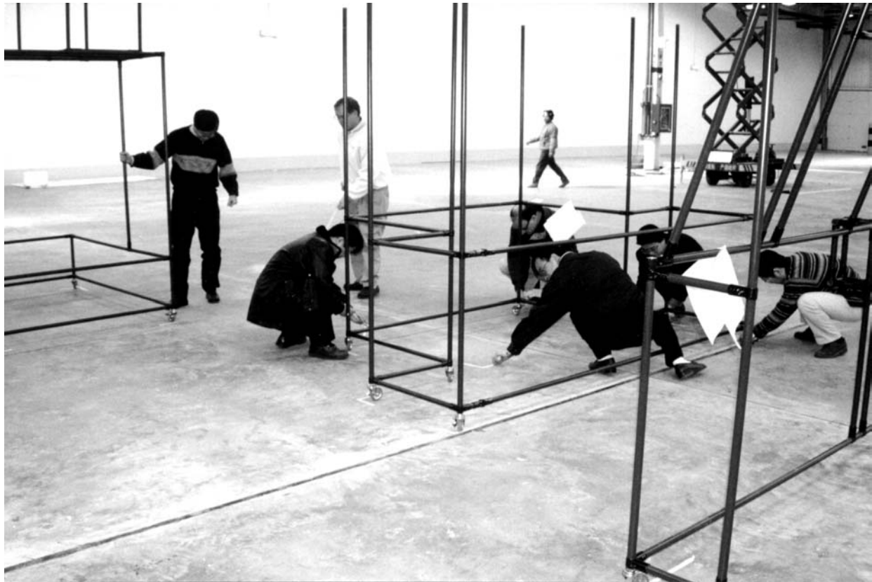
Figure 11. Physical mock-up for the gear machining cell charted in Figure 9. From the book: Planning Manufacturing Cells , © Copyright 2002 Richard Muther & Associates.
